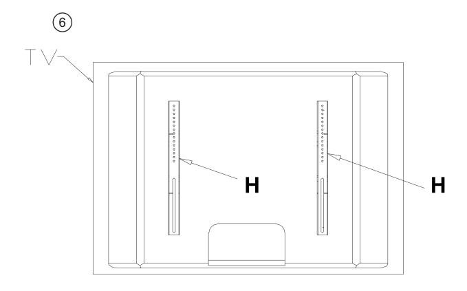
6-Fasten two TV mounting brackets(H) on the back panel of the TV. Detail assembly instructions refer to next pages.
